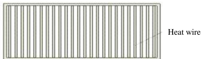
Fig.8. Cleaning roller with resistance wire heating function
